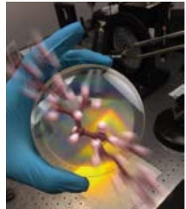
VOLUME PHASE HOLOGRAPHIC GRATING BASED ON PHOTOPOLYMERS DEVELOPED AT INAF – ASTRONOMICAL OBSERVATORY OF BRERA
