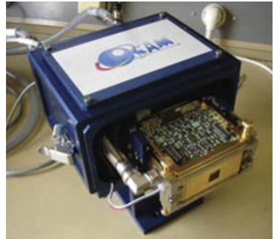
O-Cam, the worlds fastest low-noise camera, developed by OPTICON, and to be marketed
