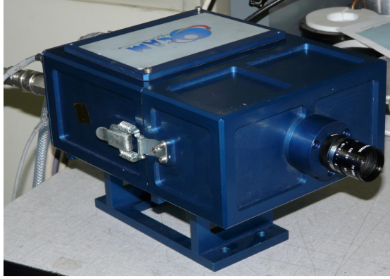
Figure 2. Left: Close-up photo of the OCam test camera. Right: Image of OCam team (Left to right: Christian Guillaume, Jean-Luc GACH, Philippe Feautrier, and Philippe Balard) taken by the OCam camera with CCD220 cold and with L3Vision multiplication gain.
